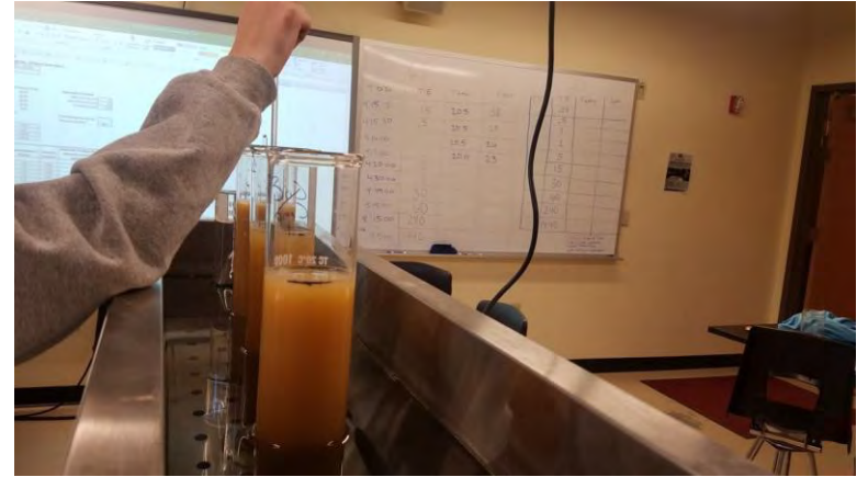
Grain Size Analysis—Hydrometer Testing
