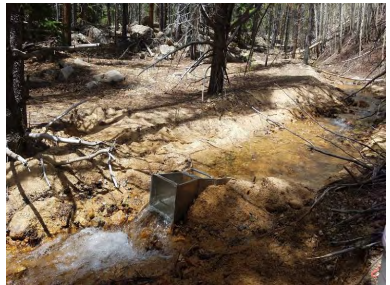
Flow Measurement at LFP-05
