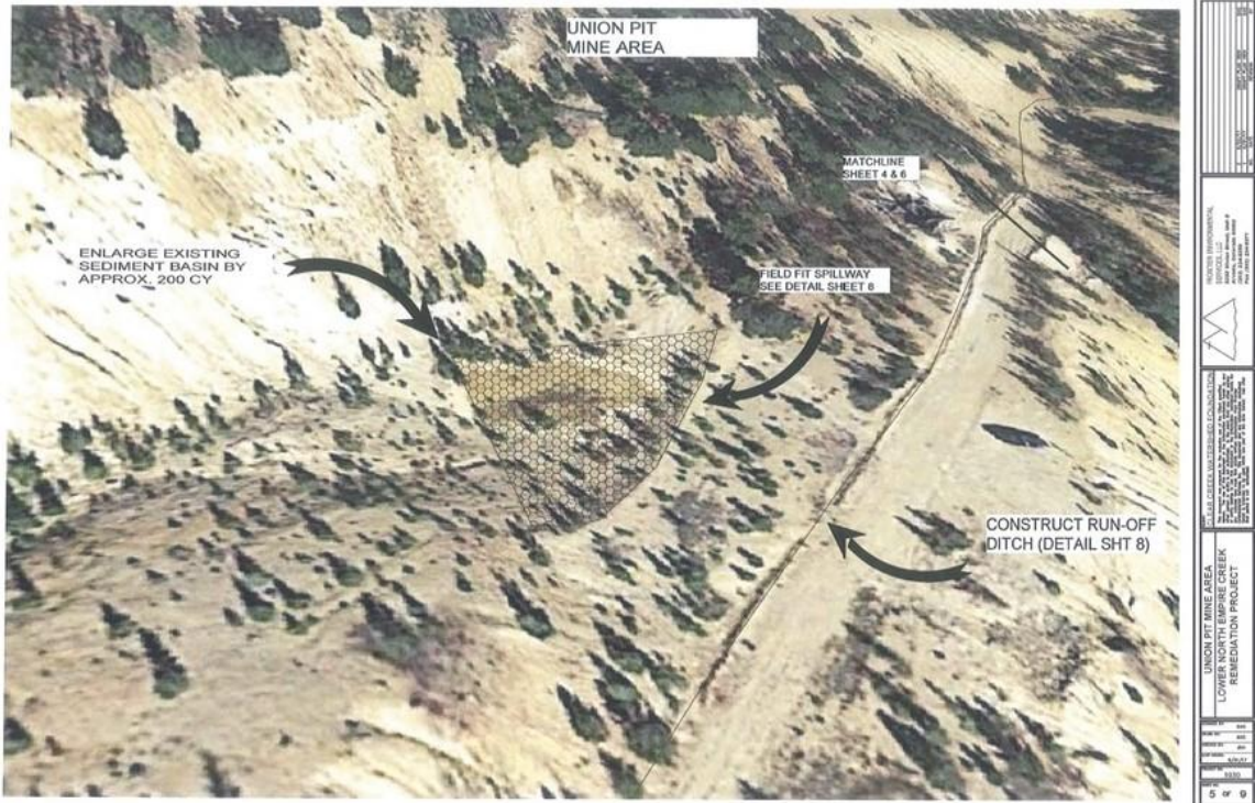
Figure 6 -Sprankle Mine Area Sedimentation Detention Basin Engineering Features
