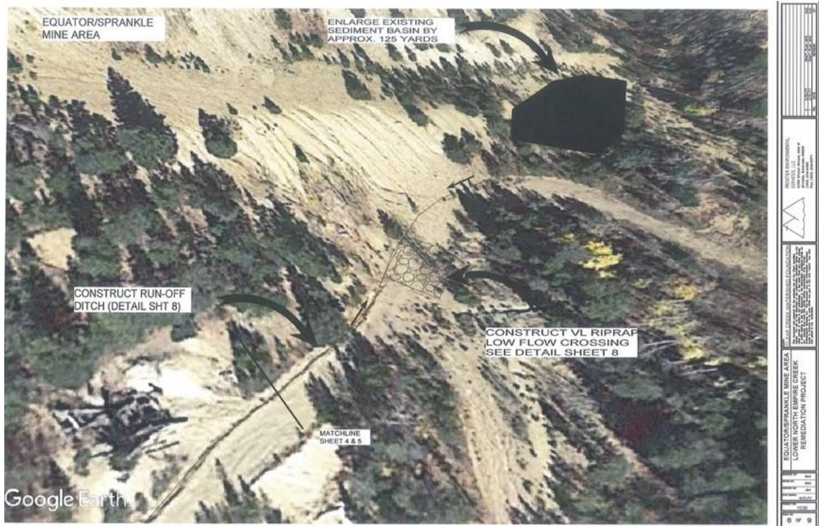
Figure 6 -Sprankle Mine Area Sedimentation Detention Basin Engineering Features
